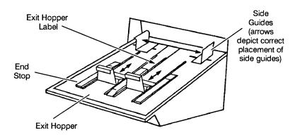
2. Adjust the End Stop of the Exit Hopper by determining the longest document to be processed. Slide the End Stop until the Arrows point to where the length of the longest document is shown on the Exit Hopper Label.
